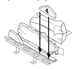
Figure 54 - Installing Log No. 4
